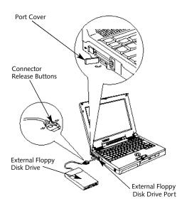
Figure 4-6 External Installation of a Floppy Disk Drive
